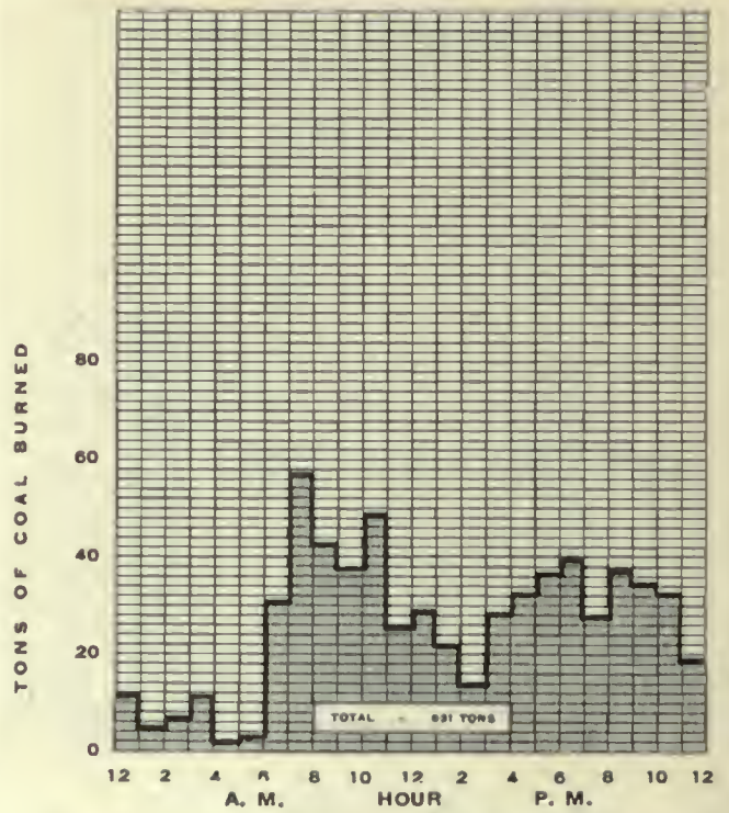
FIG. 421. DIAGRAM OF COAL CONSUMPTION. Tons of Coal Burned during the Average Day for Steam Operation in Through Passenger Service within Area of Investigation.
